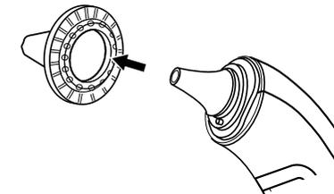
**Note:** When the probe cover is not attached correctly, the probe cover symbol “▷” will flash on the display and a measurement can’t be taken.
