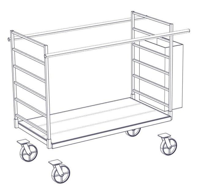
STEP 4 Attach the wheels with the nuts and bolts provided
