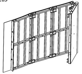
Step 3: Fold into a desire configuration for easy storage
