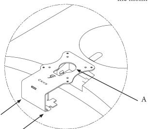
Push A from the bottom, applying equal and steady force, until hearing "click"
