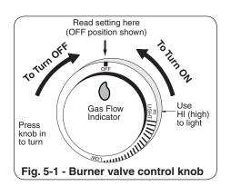
For your convenience and safety; when the control knob is turned to the ON position, the gas flow indicator will change from blue to red. (Red indicates gas flow.) See Fig. 5-1.
