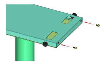
2) Place the 2 openings in the side shelf over the Allen screws, pushing the side shelf down into place. Ensure the lock and flat washers are located between the shelf and screw head. Tighten the screws with the No.5 Allen wrench.
