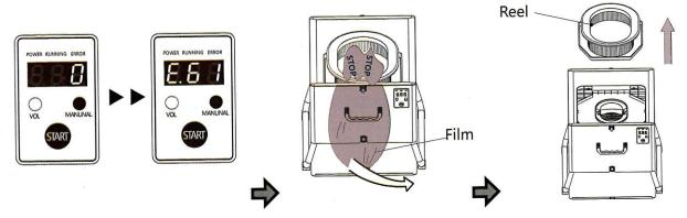
3 Place a new film roll on the main mechanism along the guide, and be sure the reflector on the film facing the detector in Main mechanism
