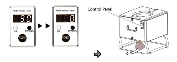
Before use the toilet, add a small bag of coagulant into the film bowl. After excretion, leave from Seat Plate, then press and hold "START" 2 seconds on the panel. The toilet starts wrapping and sealing automatically. When the speaker announces "Completed, please remove the bag.", remove the bag on the ground.
