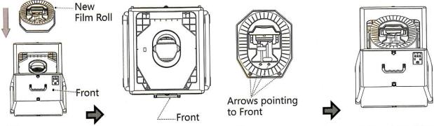
4 Move out Film Installation Tool and Film Cover, lift up the uppermost edge of film about 20cm.
