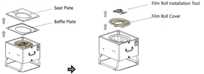
5 Pinch the outer edge of film and pull up about 20cm, then push it into the main mechanism.
