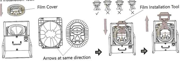
Remove Film Cover, and place Baffle Plate and Seat Plate on the toilet.
