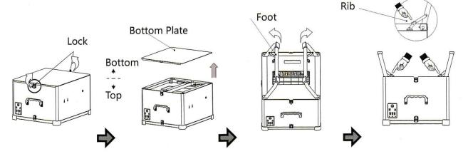
2 Overturn the product, open and move the top cover, and put the bottom plate under the product.
