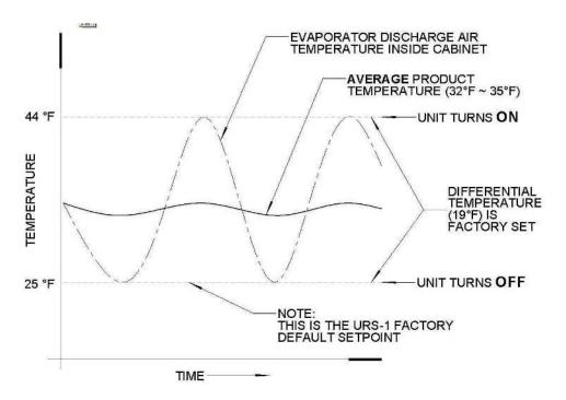
The 19°F differential is used to provide you with the best possible energy savings. A smaller differential would cause the unit to start and stop several times per hour wasting energy.
