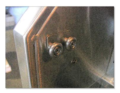
SPIT ROD SPACER LOCATED PROP-ERLY IN THE REAR HOOD ASSEMBLY AFTER INSTALLATION
