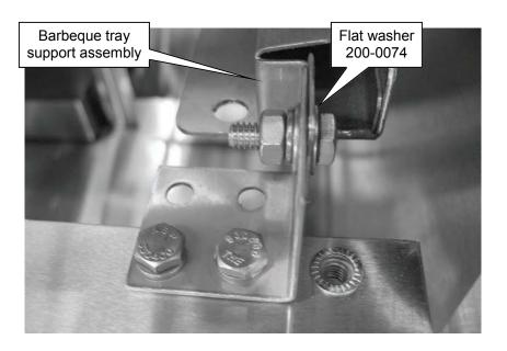
Note: The above two views show the rear left side of the barbeque being secured to the cart. To secure the rear right of the barbeque to the cart, the second mounting bracket (130-1631) must be attached in the same manner but with the bracket rotated 180°, thereby using the three holes not used when securing the rear left.
