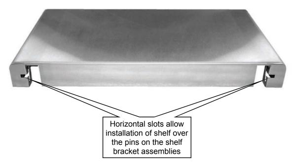
To install the shelf onto the end of the barbeque cart, hold the shelf horizontal and allowing the shelf mounting bracket pins to pass through the horizontal slots in the shelf, as shown above, position the shelf against the end of the cart then push down to engage the pins into the inner (angled) slot.
