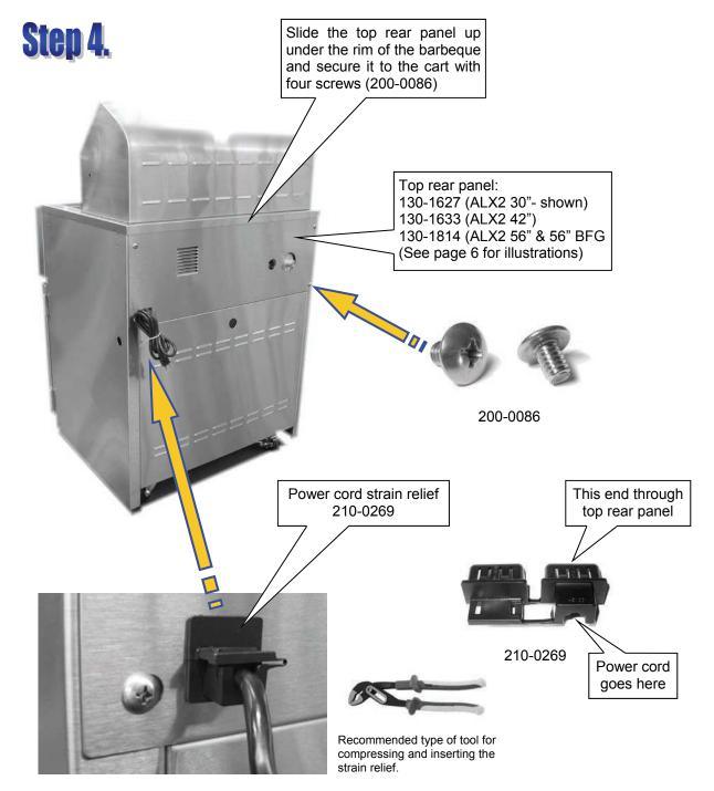
To install the strain relief on the power cord, fold the strain relief around the cord, as shown, then press the two sides together until you feel a click as the two sides lock together around the power cord. Next, insert the strain relief into the square hole and push in until the strain relief snaps into place and is locked into the top rear panel.
