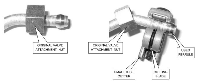
Using the small tube cutter, cut off sufficient from the end of the tube to remove the used ferrule and any damaged tube. The position of the cutter, shown above, should be suitable for leaving an adequate tube end. The large, valve attachment nut can now be removed.
