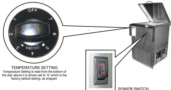
Switch the unit ON using the main ON/OFF power switch, located on the right side of the upper front panel. Check the temperature setting which has been set at the factory to #4.
