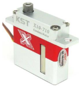
25T 5mm Output Shaft Spline
