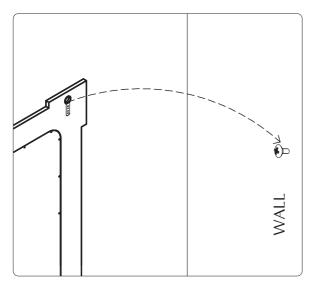
STEP 3: Lifting the mirror carefully, hook the clips on the rear of the mirror over the wall mounting anchor screws.
