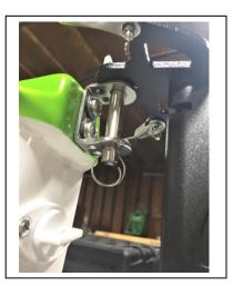
Set rudder pin into bracket and secure with ring clip. Use nylon washers as needed to take up any vertical play. Make sure it pivots freely.
