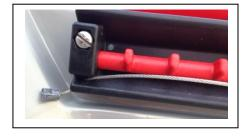
Install pivoting cable holders to rudder pivot with clevis pin and ring clip. Adjust foot braces evenly. Pull the cables rearward to eliminate slack. Run cable through cable holder and back forming a loop. Install wedge while maintaining light tension on cable. Check operation of rudder by pushing on foot braces to make sure it works evenly. Adjust cable at wedges if necessary. Install cotter pin and fold over. Cut off excess cable. Slide shrink tubing on end of cable and heat to shrink it.
