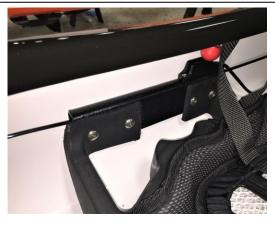
Install black rudder cable tubing from rear bosses (i.e. "frog eyes") into footrail area.
