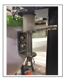
Install 1" nylon spacer onto rudder pivot pin. Set pin into bracket so that spacer is above the rudder bracket and secure with ring clip. Use nylon washers as needed to take up any vertical play. Make sure it pivots freely.
