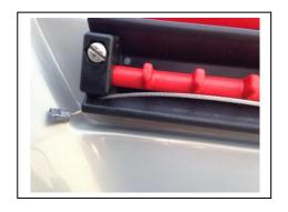
To keep footpeg upright, cut small bungee in half and attach from the front of each foot peg to the designated hole. Tie a knot at each end stretching the bungee to provide medium tension.
