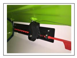
Install pivoting cable holders to rudder pivot with clevis pin and ring clip. Adjust foot braces evenly. Pull the cables rearward to eliminate slack. Run cable through cable holder and back forming a loop. Install wedge while maintaining light tension on cable. Check operation of rudder by pushing on foot braces to make sure it works evenly. Adjust cable at wedges if necessary. Install cotter pin and fold over. Cut off excess cable. Slide shrink tubing on end of cable and heat to shrink it.
