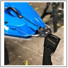
Set pin into bracket and secure with ring clip. Use nylon washers as needed to take up any vertical play. Make sure it pivots freely.
