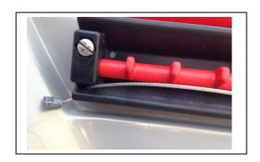
Install pivoting cable holders to rudder pivot with clevis pin and ring clip. Adjust foot braces evenly. Pull the cables rearward to eliminate slack. Run cable through cable holder and back forming a loop. Install wedge while maintaining light tension on cable. Check operation of rudder by pushing on foot braces to make sure it works evenly. Adjust cable at wedges if necessary. Install cotter pin and fold over. Cut off excess cable. Slide shrink tubing on end of cable and heat to shrink it.
