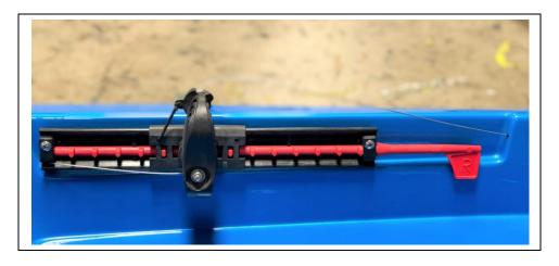
Route the cable from the rear through the tube into the cockpit area. Route the cable through the foot brace as shown in this online video -
