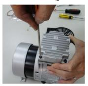
4. Open the Head Cover (part no. 18), take out the Valve Plate (part no. 16)
