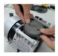
10. Replace the new Cylinder O-ring (part no. 12)
