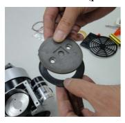
9. Hold the Cylinder in position & use a Phillips head screw driver to tighten the Round Plate Screw (part no. 10)
