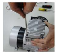
18. Replace the Cooling Fan Cover (part no.1)
