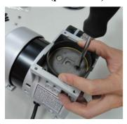
11. Replace the new Valve O-ring (part no. 17)
