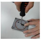
15. Put on the Valve Plate (part no.16)
