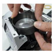
7. Assemble the new Piston Cup (part no. 8)
