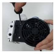
2. Use a flat head screw driver to open the Cooling Fan Cover(part no. 1)
