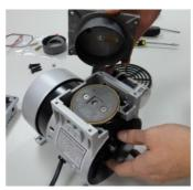
5. Use a Phillips head screw driver to unscrew the Round Plate Screw (part no. 10), Take out the Round Plate (part no. 9) & Piston Cup (part no. 8)
