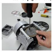
6. Replace the new Cylinder (part no. 11) in original position (note: Convex Face Up)
