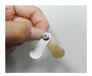
14. Reposition the Valve Fixed Strip (part no. 31) and tighten the screw .
