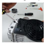
3. Use a 4mm hex wrench to unscrew the Head Cover Screw (part no. 19)
