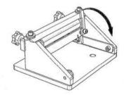
Push Roller Lever forward and insert leather strap under the blade and over the roller. Release the Roller Lever.
