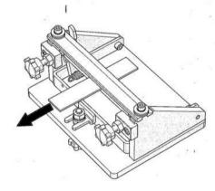
Pull the strap firmly into the blade to make the skive. Practice first on scrap leather to ensure proper thickness before working on final piece.
