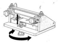
Adjust the roller height with the Vertical Adjustment Bolt to the desired thickness of the leather (after skiving). Be sure the roller is level with the blade.
