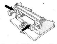
Align the cutting edge of the blade to the center of the roller by adjusting the Forward Adjustment Bolt and tighten the Lock Nut. 轉動前後調整栓,將刀刃前方對準滾輪中心,再將螺母擰緊固定。
