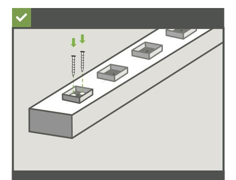
Position each spindle connector over the spindle marks you made on the rail. Ensure the connector is square to the rail.
