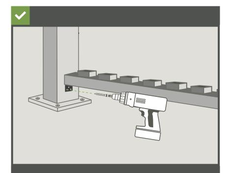
Position bottom rail so that the L bracket is on the lower side and the spindle connectors are facing up.
