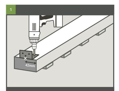
Turn the bottom rail over so that the spindle connectors are facing down.
