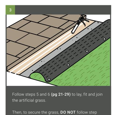
7. Instead, apply a double line of glue to the top of the haunch and use this to fix the grass to the
