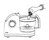
Place the bowl on the processor drive shaft and turn anti-clockwise to lock. Place the cone drive on to the food processor drive spindle.
