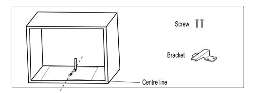
Remove the bottom cabinet template and fix the bracket with screw.
