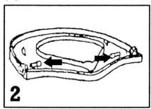
Insert 2 (F) Bushings into the appropriate holes on the seat (C) as shown.
