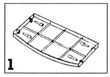
Insert 4 (F) Bushings into the appropriate holes on the Step (D) as shown.
