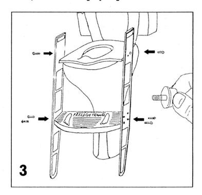
Assemble parts A, B, C and D as shown using 6 (E) screws as shown. Your FREEDOM TRAINER is now ready to use.
