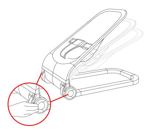
4. Do not adjust recline position when baby is in bouncer. To adjust recline position, press in button on each side of frame simultaneously and move to desired reclined position. Ensure that bouncer has locked into place and is even on each side by pressing down firmly on the seating area with your hands prior to use by your baby.
