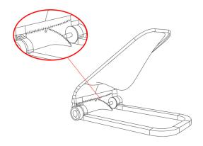
2. Pull fabric cover over and around the middle bar of the frame and zip cover closed. Bouncer seat will be tightly fitted. Ensure that zipper is fully closed and the cover is tightly fitted by pressing on seat.
