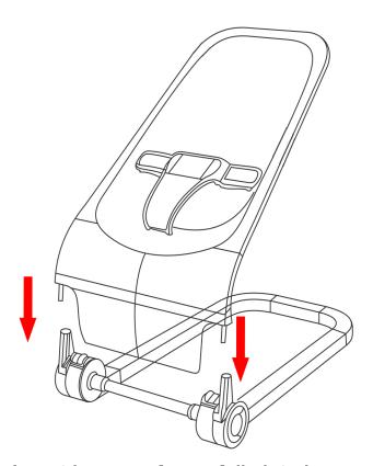
1. Insert bouncer frame fully into bouncer base on each side. Ensure that the bouncer frame is fully inserted by pushing down firmly on each side.
