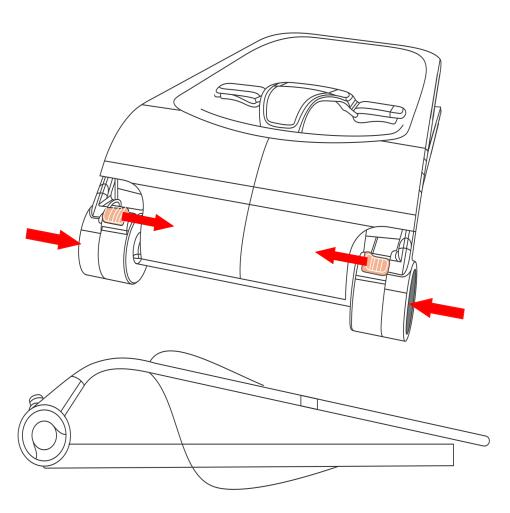
5. To store bouncer: push in both recline adjustment buttons on each side while pushing inner locks toward center to fold bouncer flat.
