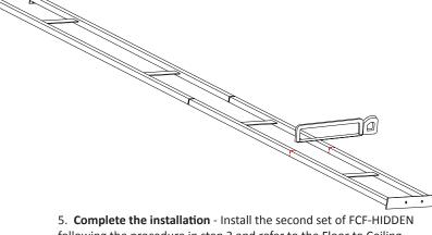
5. **Complete the installation** - Install the second set of FCF-HIDDEN following the procedure in step 3 and refer to the Floor to Ceiling Frame (FCF) installation instructions to complete the remaining installation steps, ensuring that screws are securely fastened into both mounting holes in each FCF-HIDDEN bracket.
