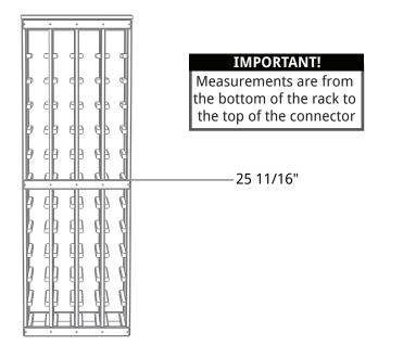
4. Flip rack over. Attach the remaining connectors to the top and bottom of the rack using the provided screws. (figure 3)
