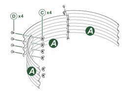
Tighten two B straight side panels with four C wingnuts and four D screws. Repeat to assemble another two B straight side panels.
