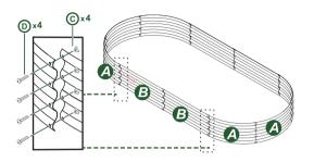
Secure four bracing rods in the 2nd connector holes.
