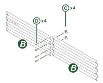
Make sure to keep the wingnuts inside and the screws outside,tighten them for reinforcement. Failure to tighten the wingnuts and screws to its maximum may cause failure
