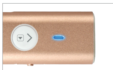
Low Battery Indicator blinks when battery is low
