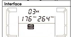
Parameter 2: Set the acceptable low voltage for bypass.
