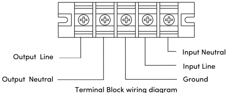
**NOTE 1:** Make sure that the wires are connected tightly with the terminals.
