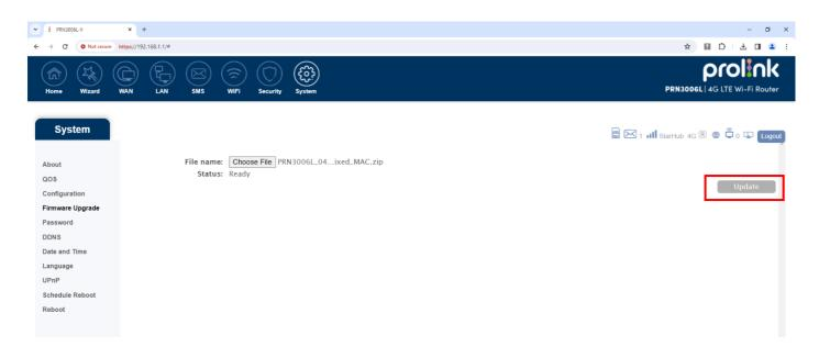
Note: Do not interrupt the update process and it is recommended to use a wired connection from the PC/laptop to do the update.
