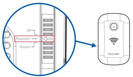
Step 2. Place the PEN1201 near your Main Router for first time setup and turn it On
