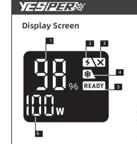
**1. Battery capacity percentage**: battery percentage of charge/discharge 2. Low current mode: support charging for the devices that need light charging current like
