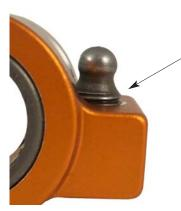
The rocker adjusters are a 7/16-20 screw with a 5/16 ball. You have to use pushrods with a 5/16 cup end. When setting pushrod length have no more than 2 and no less then 0 threads showing on the bottom side of the rocker, between the ball and rocker body. This is to make sure the pushrod contact point and rocker geometry are correct.
