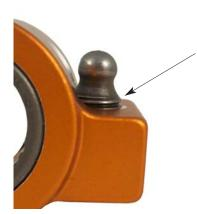
The rocker adjusters are a 7/16-20 screw with a 5/16 ball. You have to use pushrods with a 5/16 cup end. When setting pushrod length have no more than 2 and no less then 0 threads showing on the bottom side of the rocker, between the ball and rocker body. This is to make sure the pushrod contact point and rocker geometry are correct.
