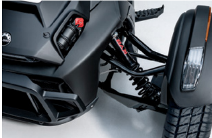
FULL KYB HPG SHOCKS Front and rear KYB HPG shocks with remote adjusters and 1 inch of extra suspension travel to optimize your ride and improve comfort.
