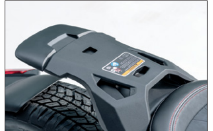
MAX MOUNT STRUCTURE Makes the unit 1+1 ready. It also increases the carrying capacity for different storage options.
