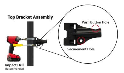
Install top banner arm into the bracket making sure the push button is engaged through the top hole in the bracket.
