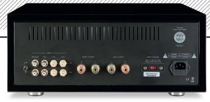
**ABOVE:** No 'digital' here – just one MM phono and three line inputs on RCAs with single sets of switched speaker outputs on 4mm sockets/binding posts
