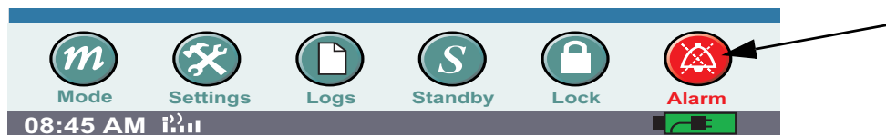
Figure 152: Low Battery Alarm button
