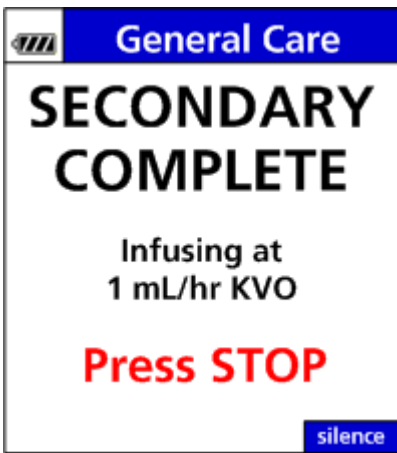
Figure 44. Secondary Completion; KVO Alarm
