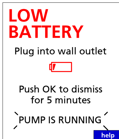
Figure 66. Low Battery Alarm
