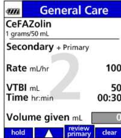
Figure 41. Secondary Infusion Setup Screen
