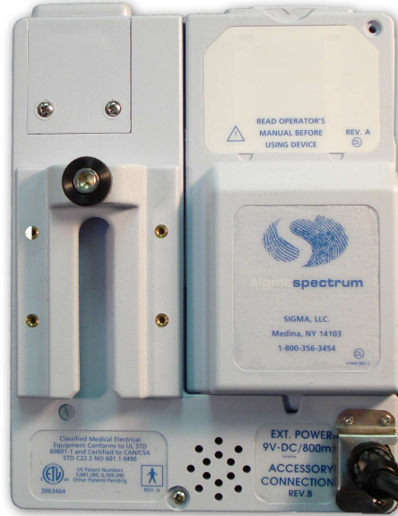
Figure 4. Back View- With Standard Battery (P/N 35724)
