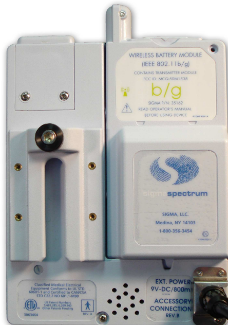
Figure 6. Back View- With 802.11b/g Wireless Battery Module (P/N 35162)
