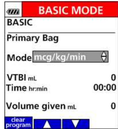
Figure 33. Arrow Soft Keys used to scroll through Dose Rates
