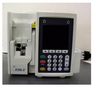
The Plum A+ Infusion System is designed to meet the fluid delivery requirements of today's evolving healthcare environments. It is a cassette based multi-function infusion system. The Plum A+ allows two lines in and one line out. The pump can be used for standard, piggyback, or concurrent delivery. Therapy modes include:
