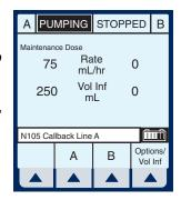
17) The user should acknowledge the Callback message and stop the audio alarm by pressing (SILENCE).
