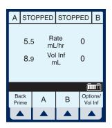
2) Select and hold ▲ [BACK PRIME] until fluid pumped from line A to line B has expelled the air from cassette air trap into Secondary container.
