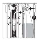
**CAUTION:** Ensure all four cassette latches are clearly visible after the cassette is installed. Refer to Loading the Cassette on page 32.
