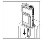
Note: The docking station light is yellow while the docking station is charging. When the docking station is fully charged, the light is green.
