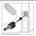
**2** Plug the printer cable into the printer port on the rear, right side of the docking station.
