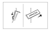
**2** Push down on the cassette release (large black button) on the top of the pump.
