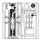
**CAUTION:** Ensure all four cassette latches are clearly visible after the cassette is installed. Refer to Loading the Cassette on page 32.
