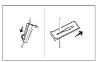
**3** Press the cassette release button to eject the cassette from the pump.
