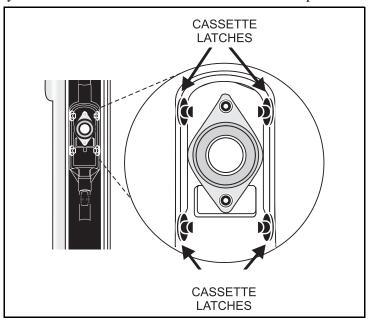
Line up the cassette as shown (with the flow stop button facing the pump).
