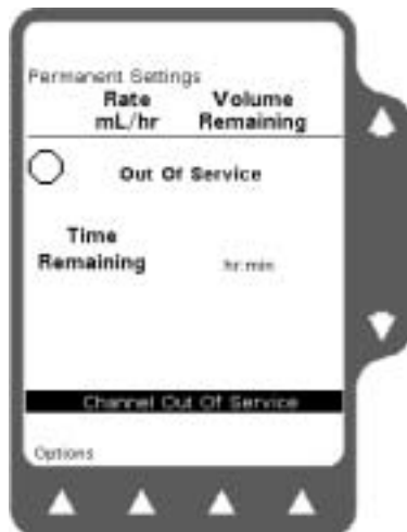
Figure 6-11 Channel Failure Display
