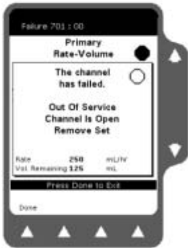
Figure 6-10 Channel Failure Pop-up Message
