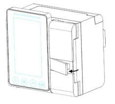
(3) Gently pull the infusion tube, straighten it, and fix the infusion tubing the tube groove at both ends from top to bottom, and close the antifree flow clip to clamp the infusion tube. (2)Push the anti-flow free clip to the lower
