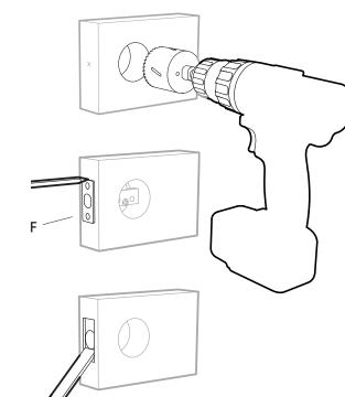
3 Install Enclosed Latch and Strike Plate
