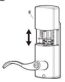
This Electronic lock requires (4) High Quality AA Alkaline batteries. When all 4 batteries are installed in the correct position, you should hear 2 beeps and the keypad will illuminate.
