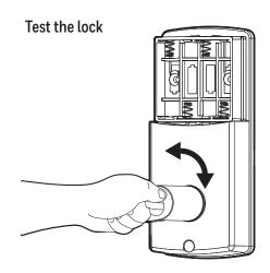
Lock and unlock using the knob make sure the latch is opening and closing easily. If not, go back to step 2 and ensure you followed the steps
