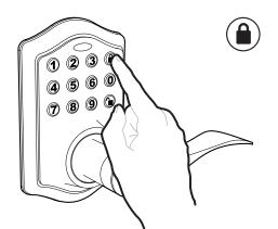
Test unlocking Press 1-2-3-4-
