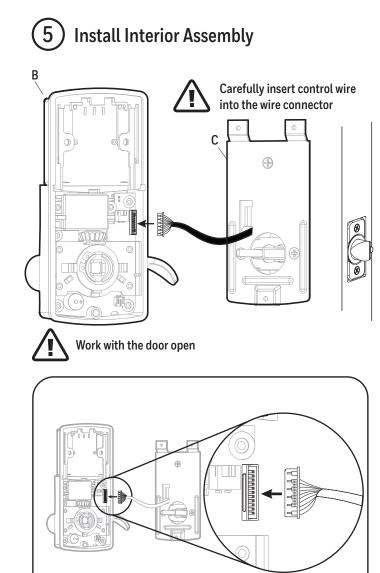
NOTE: Make sure the connector dots line up with the dots on the wire
