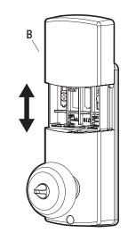
This Electronic lock requires (4) High Quality AA Alkaline batteries. When all 4 batteries are installed in the correct position, you should hear 2 beeps and the keypad will illuminate
