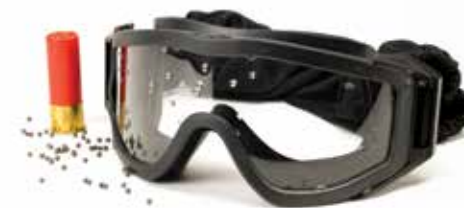
Loadout ballistic goggle shot with 12 gauge shotgun and 2 3/4 inch steel #6 at 25 yards.
